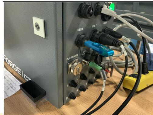
**Note:** You must insert a USB flash drive into the Forge Controller to import or export tasks. The features will not be accessible unless a USB is detected.
