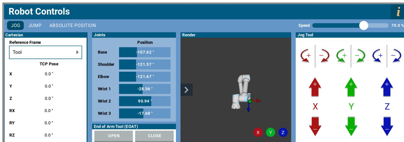
There are three types of motion the RCP can instruct the robot arm to do: *jog*, *jump*, and *absolute position*. There are three tabs on the RCP, each corresponding to a type of motion for the robot arm and each including options for Cartesian and Joint motion. The 3D rendering, speed slider, and frame selection are present on all three tabs.
